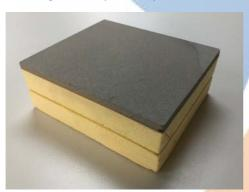
The jointing between the panels is to include a 3-5mm gap sealed with a 10mm backing rod and appropriate silicon sealant. Where a 10mm gap is provided for the egress of any water, an appropriate bushfire weephole protection or equivalent is to be installed.
